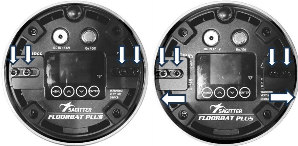
**5.** Turn the projector over again, bringing it back to the position with the LEDs facing upwards and insert the M4x8 locking knob through the hole in the cover, screwing it onto the respective M4 hole of the projector. In this way, the safety of the cover itself against accidental release is guaranteed.
