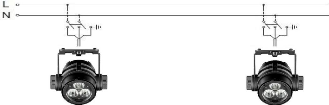
When the projector is powered by the mains with its specific external adapter, it must be connected to a power supply system with a proper earth system. Moreover, it is recommended to protect power supply lines of the products from indirect contact and / or shorting to earth by using appropriately sized anti electrical shock switch.
