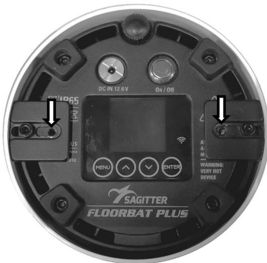
2. ... remove the 2 internal screws of the 4 that block the mobile brackets.
