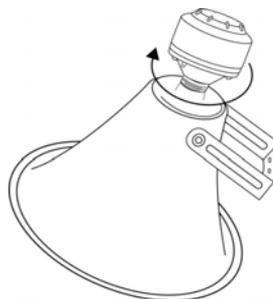
2. Firmly fix the bracket in the place where you want to mount the horn.
