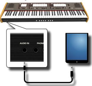
Use the AUDIO IN knob to adjust the input level the CLASSICO L3's AUDIO IN jack to the output of the signal received.
