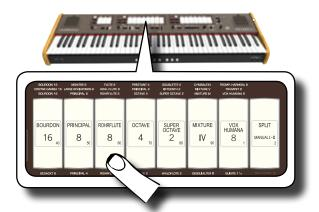
In the example above we select a register in the MANUAL I division. The tilt tab flashes to indicate that we are in edit mode.
