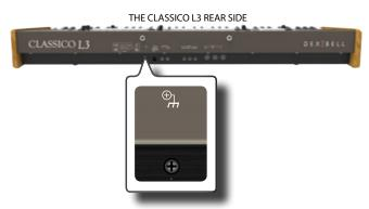
Use the screw-type ground terminal to connect to ground or to connect to the chassis of the mixer, preamp, or other device in your system.
